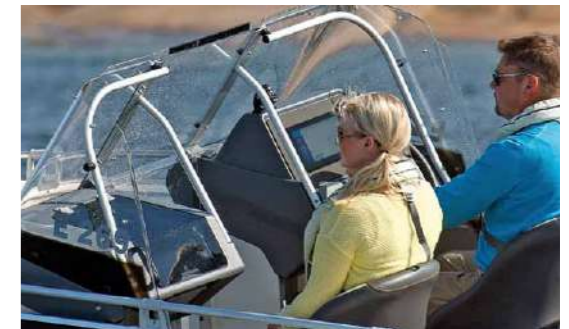
The fixed door between the consoles gives protection from wind and spray
