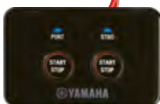
3 - TWIN ENGINE START / STOP SWITCH
